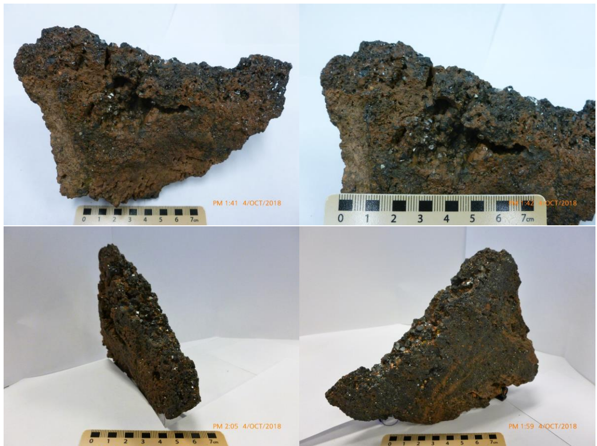
Figure 4: Photos taken of the “diktytaxitic” magnetite sample EL-BM-03.
