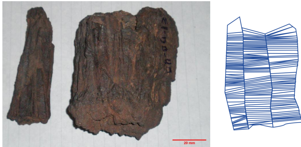
Figure 6 & 7: (left) Another photo of a “columnar” magnetite sample not used in this study, but with a more defined texture; (right) Sketch of the texture in question.
