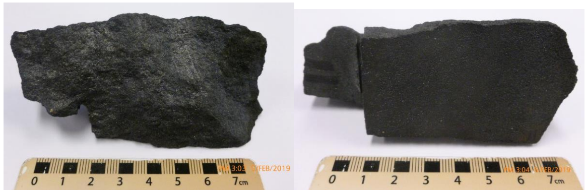
Figure 9: Photos taken of the magnetite “welded tuff” sample EL-JM-11.
